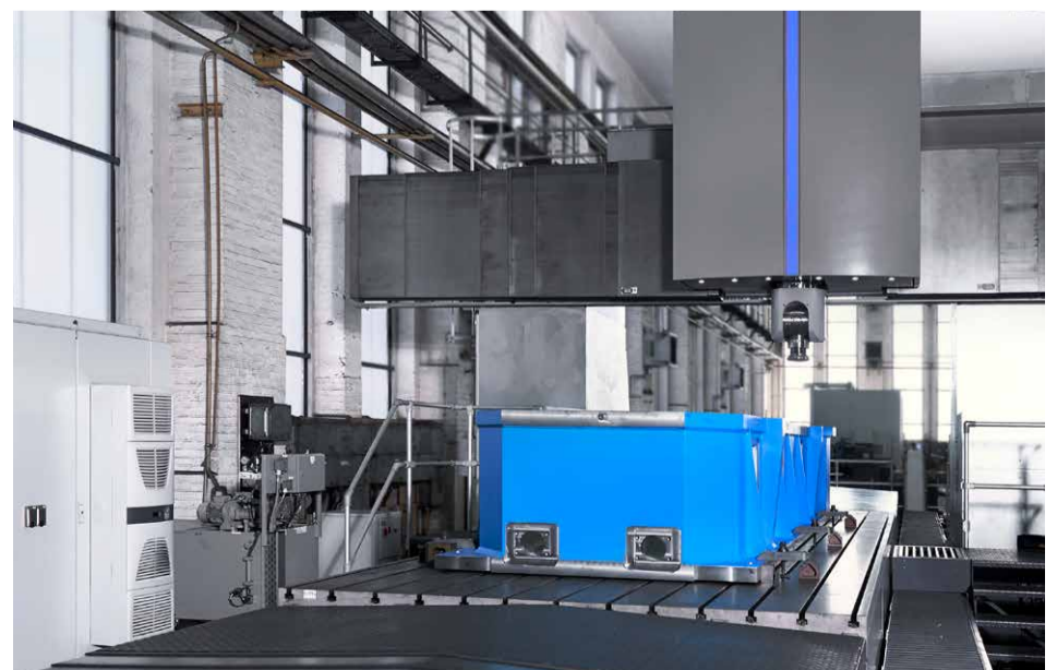
The ProfiMill compact machines the housing of an XXL helicopter test bench gearbox
